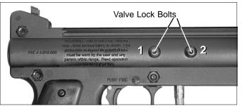
Reinstalling: Apply red loctite to bolts threads when reinstalling. Do not over tighten valve lock bolts when reinstalling.
