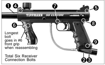
To remove the left-side receiver, unscrew bolts (4-9) receiver connection bolts. Then carefully lift the left-side receiver to access the internals.
