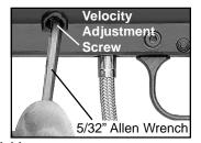
To adjust the velocity use the 5/32" allen wrench included with your marker. The velocity adjustment screw is located on left side receiver. To adjust the velocity down, turn the screw inward or clockwise. To turn the velocity up, turn the screw out or counterclockwise. Do not remove velocity screw.
